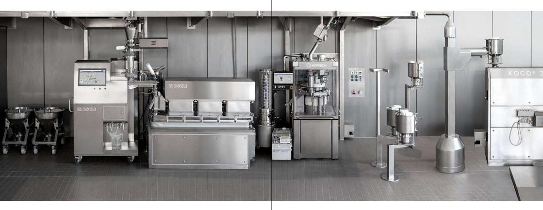
Continuous process technology continues to gather momentum in the pharmaceutical industry. KORSCH has partnered with L.B. Bohle and a consortium of technical specialists on a fully integrated continuous process line which incorporates NIR technology and a fully integrated supervisory control system.
