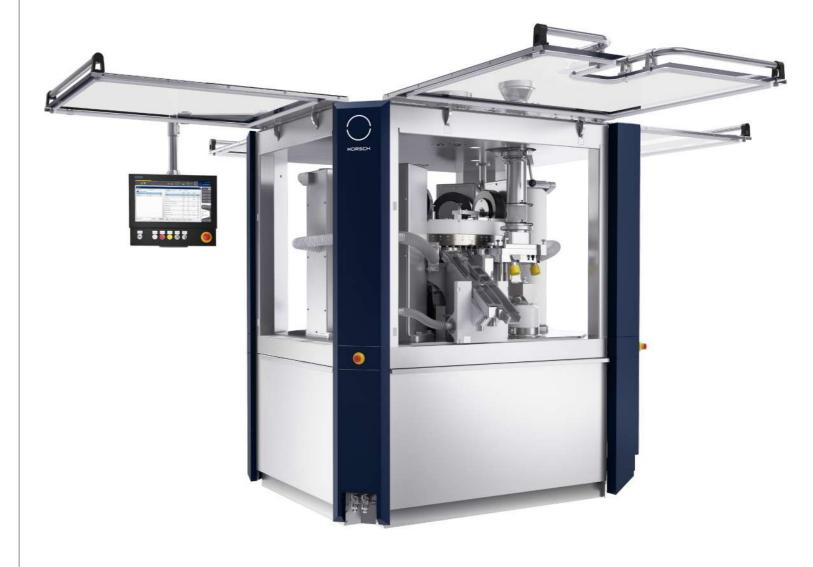
The XT 600 has the flexibility to produce both single- and bi-layer tablets with a maximum output of 1,380,000 single-layer and 414,000 bi-layer tablets per hour. A bi-layer conversion kit can be adapted to the machine at any time, which includes the components to ensure individual layer weight control, first-layer sampling, and absolute separation of product layers.
