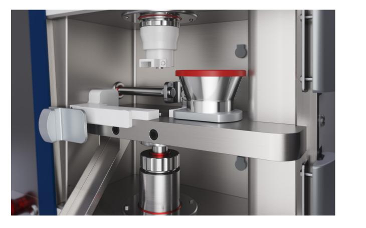
The STYL'ONE Nano is equipped with a powerful data acquisition system capable of recording multiple signals from both upper and lower punches, including pre- and main compression forces, punch displacement, and ejection force. In addition, the instrumented die captures maximum and residual die wall pressures, enhancing material characterization and formulation understanding.
