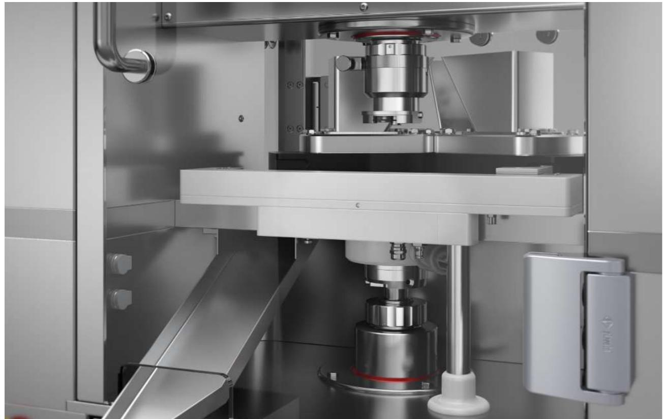
The STYL'ONE Evo is equipped with a powerful data acquisition system capable of recording multiple signals for both upper and lower punches, including pre- and main compression forces and displacement. High frequency acquisition allows the capture of very short events, such as ejection and take-off. In addition, the instrumented die records maximum and residual die wall pressures, enhancing formulation understanding.
