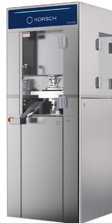
Thanks to its powerful drive system and advanced instrumentation, the STYL'ONE Evo precisely controls punch displacement, enabling the execution of a wide range of compression cycles, including V-shape and extended dwell-time, as well as roller compactor and rotary press profiles.
