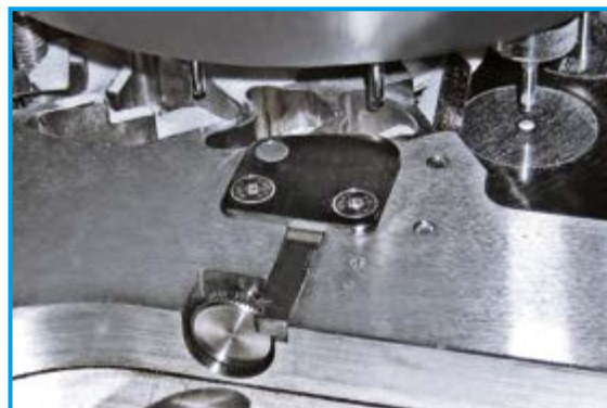
XL 100 with Compression Force control and single tablet rejection
